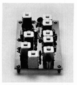
Whf converter board for the fm receiver. Although designed for use with the 10.7 MHz i-f/audio board, it can be used with other i-f systems as discussed in the text.
